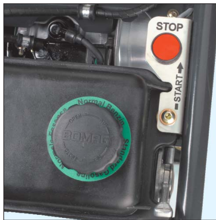
Operational safety: engine stop switch integrated into the handle.
