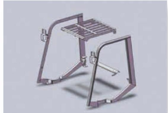
The triplex plate overhead guard is developed using three pieces: left side, right side and top canopy making replacement, when appropriate and authorized, more convenient
