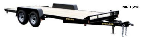
Built to last, these trailers are ideal for agricultural and landscape use. Designed with fenders outside of a full width, low profile deck, these trailers allow maximum space for loading.
