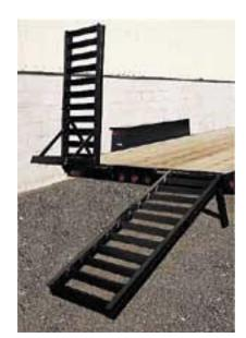
Ramps are engineered for easy return to storage position after loading.
