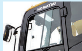
Remote intermittent wiper with windshield washer
