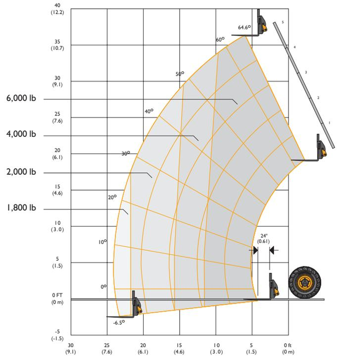
This load chart is for the rated capacity of the machine with 66" wide standard carriage and 48" pallet forks. Use only JCB approved attachments and check the relevant load chart for the machine model. If in doubt, consult your dealer. If the load rating of the machine differs to that of the attachment, the lower rating becomes the overall capacity.
