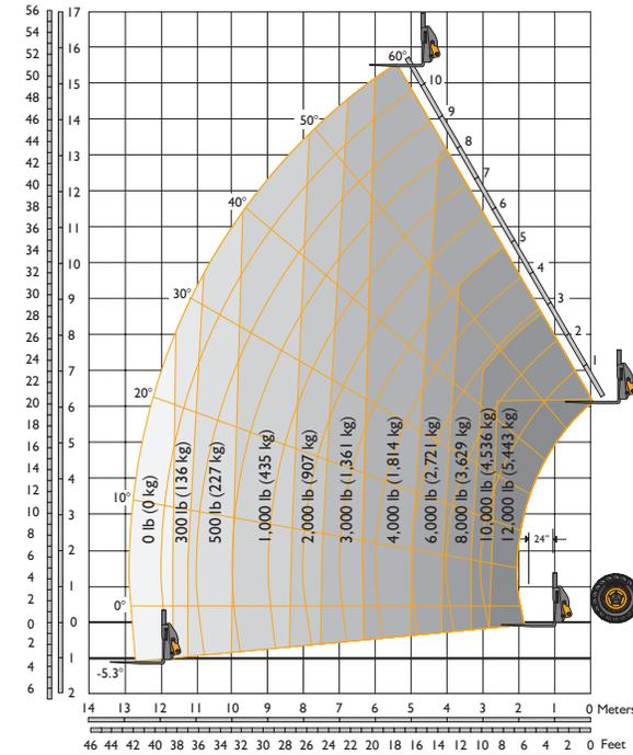
These load charts are for the rated capacity of the machine with 72" wide standard carriage and 48" pallet forks.
