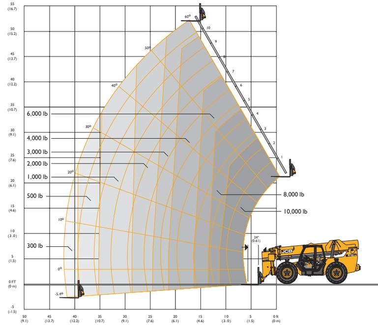
These load charts are for the rated capacity of the machine with 66" wide standard carriage and 48" pallet forks. Use only JCB approved attachments and check the relevant load chart for the machine model.
