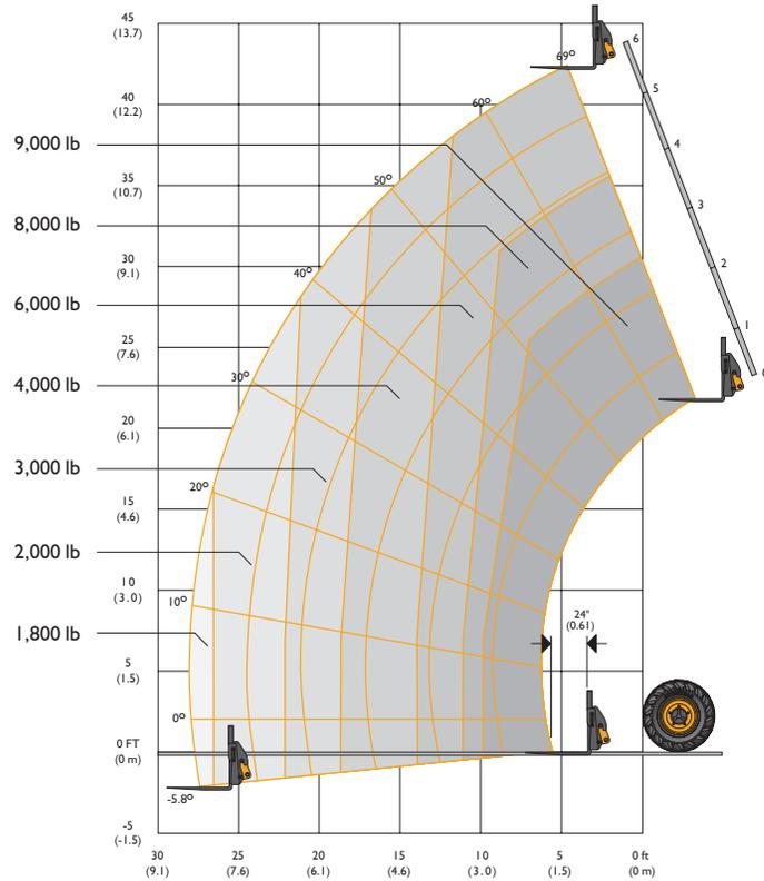
This load chart is for the rated capacity of the machine with 66" wide standard carriage and 48" pallet forks. Use only JCB approved attachments and check the relevant load chart for the machine model. If in doubt, consult your dealer. If the load rating of the machine differs to that of the attachment, the lower rating becomes the overall capacity.
